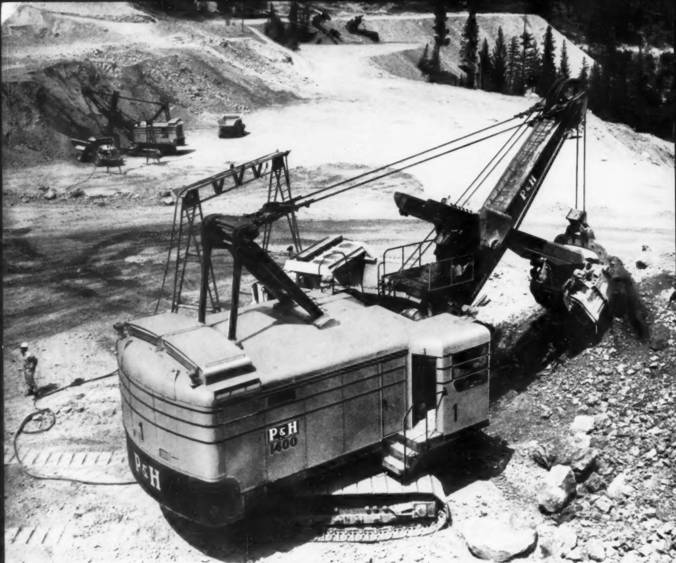
4½-yard P&H Electric working at Craigmont Mines Limited's new mine near Merritt, B.C.
